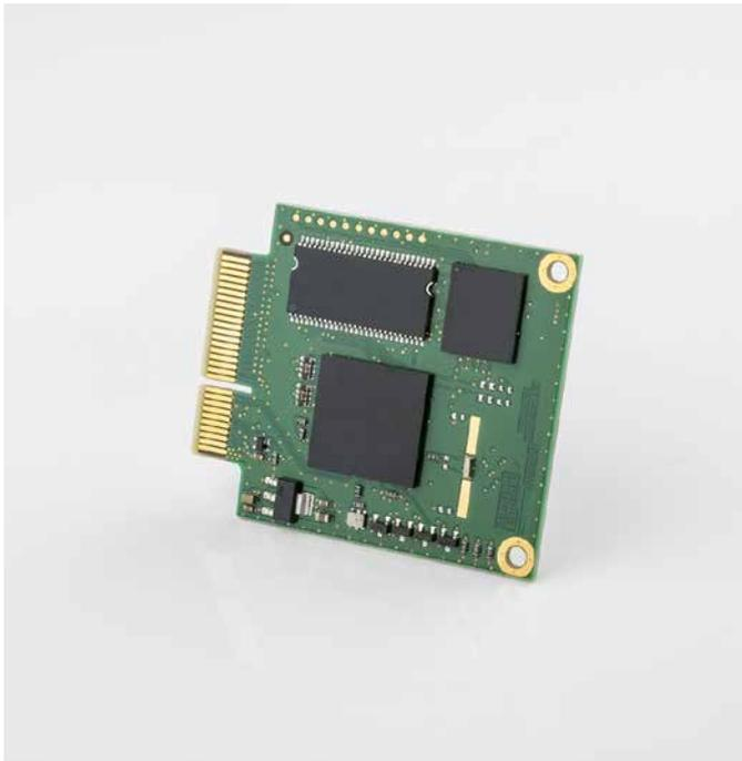
The µModule card is based on the hardware of the StarGraph card but has no connectors.
